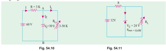
**Example 54.7.** A 24-V, 600-mW Zener diode is to be used for providing a 24-V stabilized supply to a variable load (Fig. 54.11). If input voltage is 32 V, calculate the (i) series resistance R required (ii) diode current when  $R_L = 1200 \Omega$ . (Applied Electronics, Punjab Univ. 1991)
