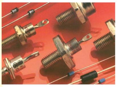
A major application for zener diodes is voltage regulation in dc power supplies. Zener diode maintains a nearly constant dc voltage under the proper operating conditions.
