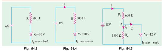
**Solution.** Polarity-wise, the diode is properly-biased. Since applied voltage is greater than  $V_z$ , the diode is properly voltage-biased.
