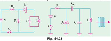
proper current level for it. The capacitor  $C_C$  is the coupling capacitor. As the switch S is closed, the diode is set into oscillations whose frequency equals the resonant frequency of the tank.
