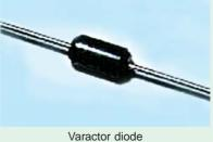
The hyperabrupt-junction diode has highest impurity concentration near the junction. It results in narrower depletion layer and larger capacitance. Also, changes in  $V_R$  produce larger capacitance changes. Such a diode has a tuning range of 10 : 1 enough to tune a broadcast receiver through its frequency range of nearly 3 : 1.
