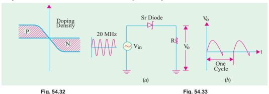
Fig. 54.33 (*a*) shows a step-recovery diode being driven by a 20-MHz signal source. As seen from Fig. 54.33 (*b*), it conducts in the forward direction like any diode. During the reverse half-cycle, we get reverse current due to the draining of the stored charge after which current suddenly drops to zero. It looks as though diode has suddenly *snapped open* during the early part of the reverse cycle. That is why it is sometimes called a *snap diode*.
