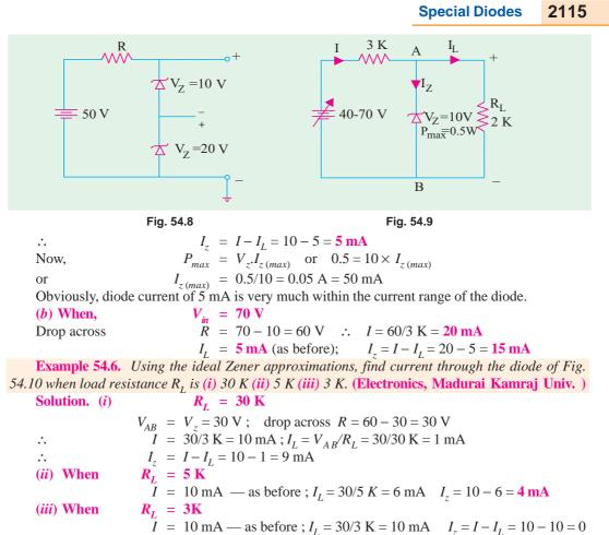
In this case, it is obvious that the diode is just on the *verge of coming out of breakdown region*. If  $R_L$  is reduced further, the diode will come out of breakdown region and would no longer act as a voltage regulator.
