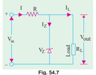
The load resistance  $R_L$  across which a constant voltage  $V_{out}$  is required, is connected in parallel with the diode. The total current *I* passing through *R* equals the sum of diode current and load current *i.e.*  $I = I_z + I_L$ .
