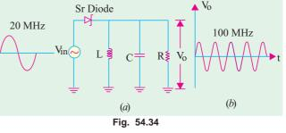
Fig. 54.34 shows how the output of a step recovery diode can be
