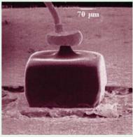
Discrete commercial Si tunnel diode
